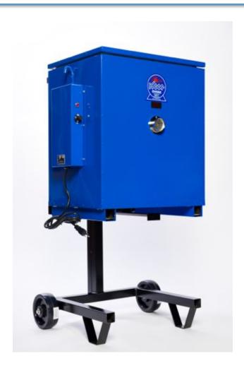
Purpose: To keep subarc welding flux dry
