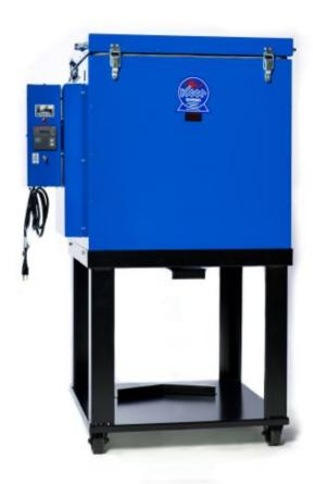
Purpose: To keep subarc welding flux dry
